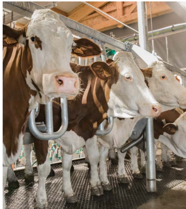
Gentle spring loaded sequence gates guide each cow from the wide entry area into its own comfortable milking stall.
