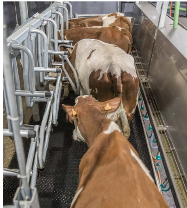
Gentle spring loaded sequence gates guide each cow from the wide entry area into its own comfortable milking stall.
