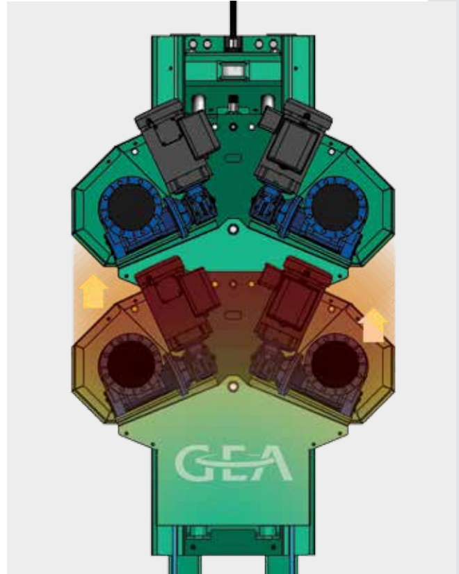
The Fit R-300 drive unit moves upward one side after the other, along the two guide pillars, until it reaches the end of its stroke.
