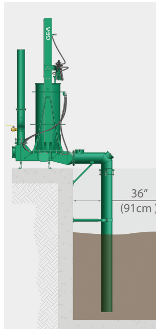
Installation on the floor next to the reception pit Suction pipe 36" (91 cm) from the wall. The pump must be installed in a recess when the reception pit is deeper than 10 feet (3 m).
