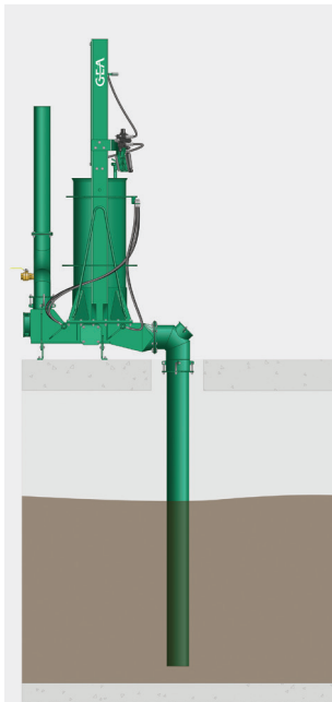
Installation on the floor above the reception pit Suitable for a reception pit with a depth of 10 feet (3 m) maximum.
