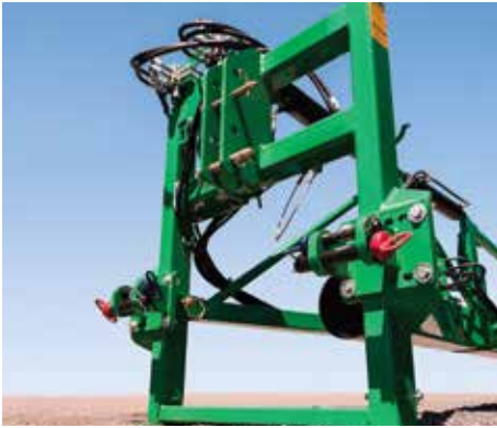
Optional 3-point Quick Hitch For easy coupling of pump to tractor.
